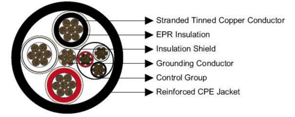
**Conductors:** Stranded annealed tinned copper conductor.
